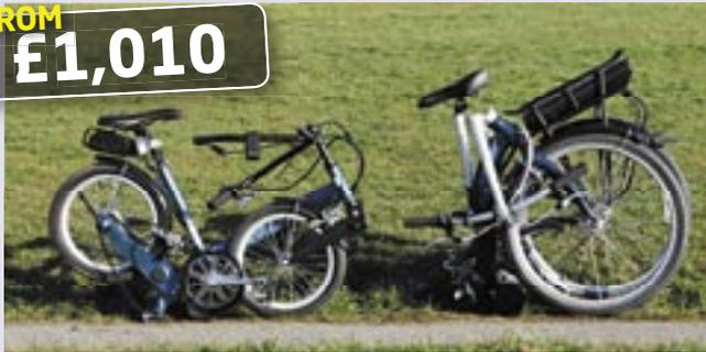
This is the only kit available in the UK (we're aware of) that drives through the bike chain; generally a more efficient system and often associated with companies producing extremely well-engineered products, as with Sunstar. This clever system fits almost any bike, effectively replacing pedal axle and chainwheel.
